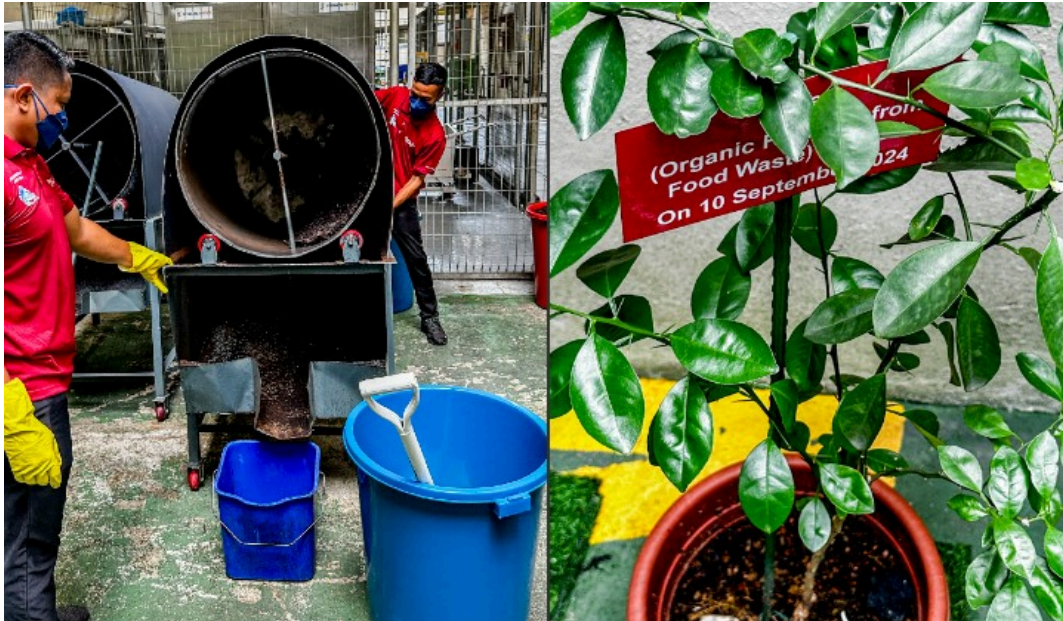
From food scraps to fertiliser — Pavilion Bukit Jalil's trommel screener processes composted food waste into organic fertiliser, nurturing the very plants you see growing in the mall today. Waste nothing. Grow everything. (Pix: Fernando Fong)
